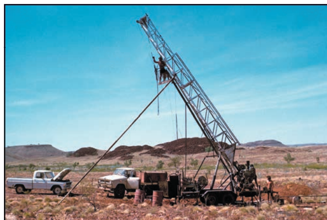
Figure 34. Drilling to prove nickel reserves at Whundo.
