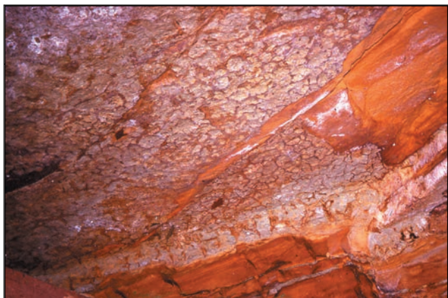
Mudstone bed with mudcracks seen in section and from the underside, in the roof of a stope in the Engine Vein mine.
