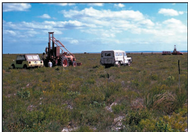
Figure 24. Drilling to prove the ilmenite-rich heavy mineral sands at Eneabba.
